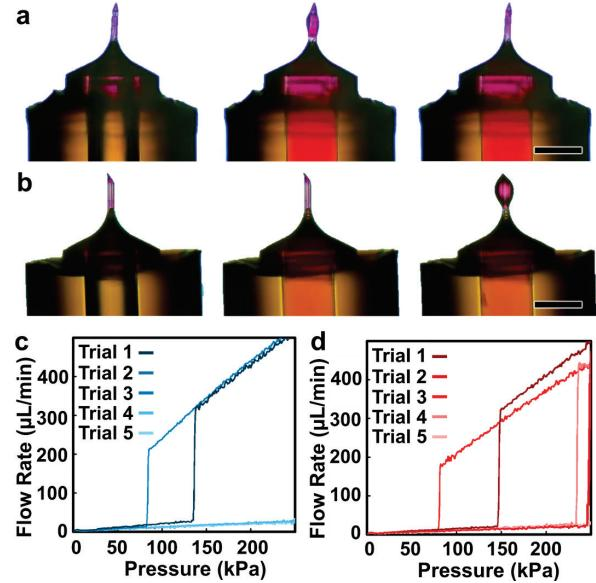
**Figure 3:** Experimental results for **(a, b)** infusion of Rhodamine B-dyed IPA through the microneedles and **(c, d)** microfluidic burst pressures corresponding to the **(a, c)** architecturally complex and **(b, d)** control designs. Scale bars = 100  $\mu\text{m}$
