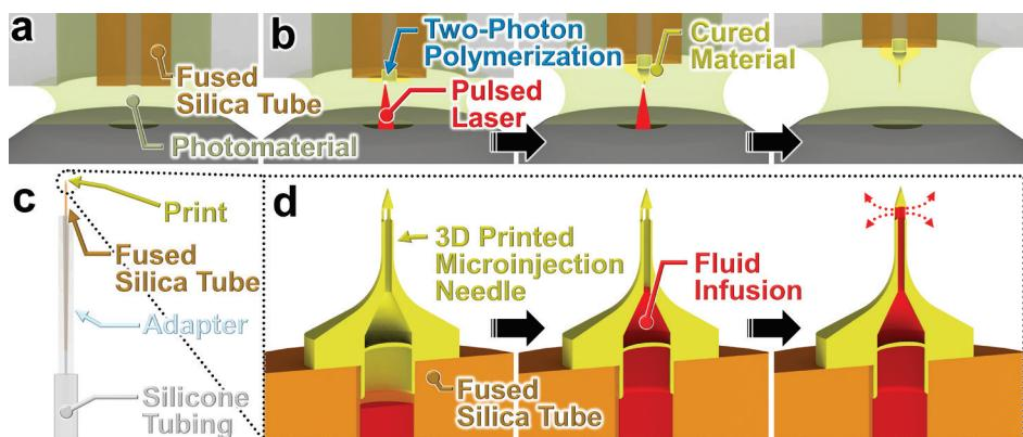
**Figure 1:** Illustrations of “*ex situ* Direct Laser Writing (*esDLW*)”-based microinjection needles. (a) A macroscale tube mounted in the 3D printer. (b) Point-by-point, layer-by-layer scanning of a tightly focused pulsed IR laser to initiate two-photon (or multi-photon) polymerization. (c) Assembly configuration for fluidic loading. (d) Fluid infusion process through an *esDLW*-printed architecturally complex 3D microneedle design.
