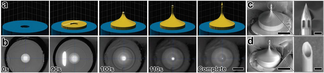
**Figure 2:** Fabrication results for esDLW-based printing of microinjection needles. **(a)** Computer-aided manufacturing (CAM) simulations and **(b)** corresponding sequential micrographs of the esDLW 3D printing process. **(c, d)** SEM micrographs of printing results for **(c)** architecturally complex and **(d)** control microneedle designs. Scale bars = 100  $\mu\text{m}$  (insets = 10  $\mu\text{m}$ )
