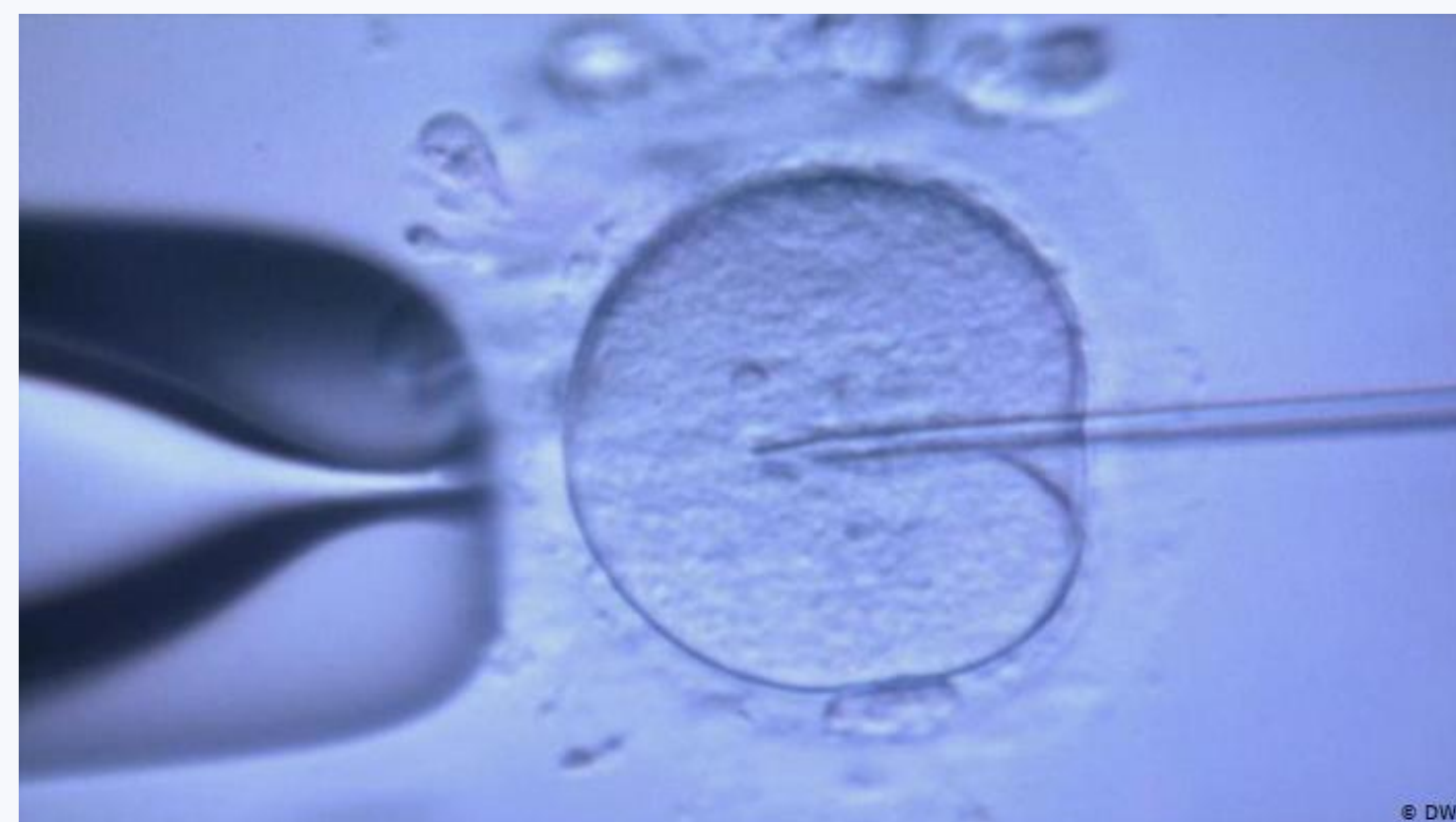
Figure 1: Injection into egg via industry standard needle. A clear, glass microcapillary is used to inject sperm into egg sample during the IVF cycle. The needle is transparent and the tip of the capillary is likely to get clogged with proteins, increasing variability per injection.
