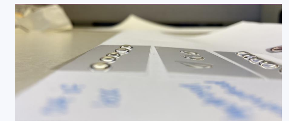
Figure 7: Eye level view. Out of box/untreated and hydroxyl activated (top). Aminized/Silanized and PEG functionalized (bottom)
